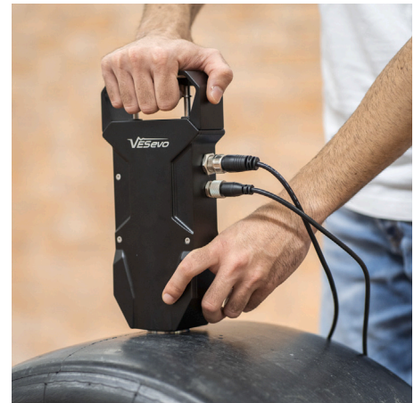
Fig. 5. VESevo device in operation for testing a high-performance tire.
