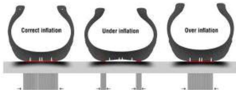
Figure 13 Inflation pressure effects on the contact patch
