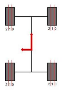
Tires start the simulation at a global temperature of 65°C, while air temperature has been set at 15°C, and road temperature at 15°C. Starting inflation pressure is hypothesized at 1.3 bar for the four tires.
