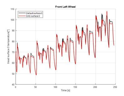
In the first plot, the comparison between tread external temperature (in particular, on rib 0 for front left wheel) in the two cases is observable. Due to the reduced friction power (the product between the tangential force and the sliding speed), linked to the decrease of tire slip angle in the D.A.S. activation phases, the simulation with the device leads to a lower thermal level.
