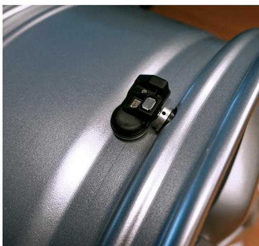
**Figure 7.** TPMS sensor to measure pressure and temperature inside the tire.
