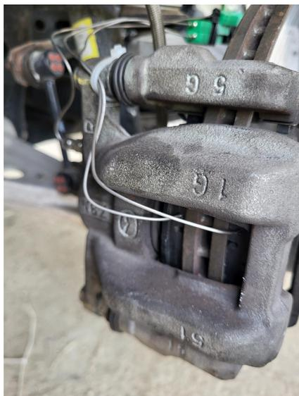
**Figure 4.** Thermocouples installed to acquire temperatures of disc and brake pad.
