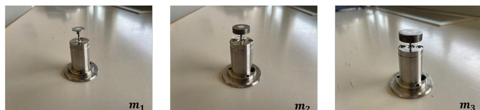
**Figure 14.** Sensor modules with the newly designed masses and springs.
