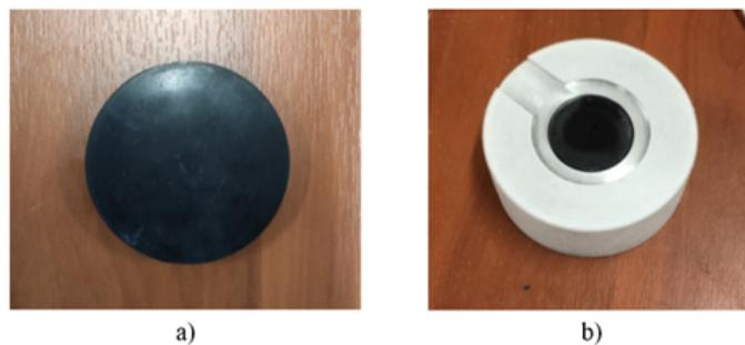
**FIGURE 11.** (a) 40 mm diameter compound specimen; (b) Specimen in the suitable holder for testing
