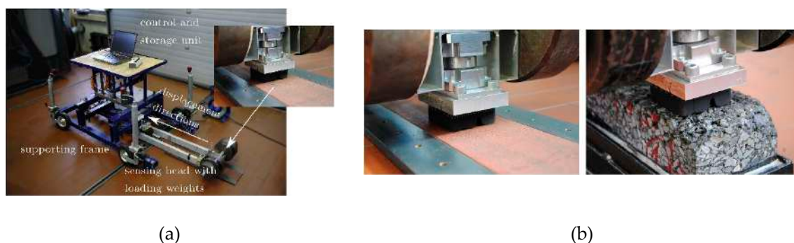
Figure 21. (a) LiRep general view (left); (b) detail of two different road surface configurations [70].
