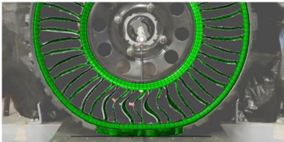
**Figure 9.** Comparison of the deformed shapes.
