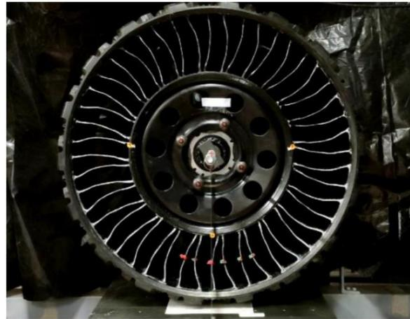
**Figure 4.** NPT setup for DIC tool.
