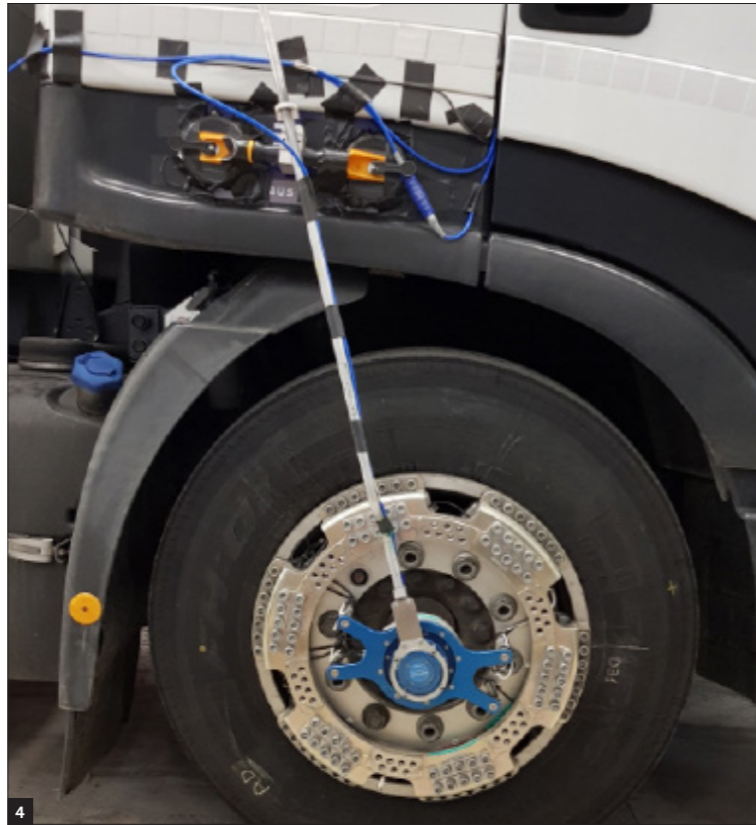
Figure 4: Front and rear were fitted with dynamometric wheels
