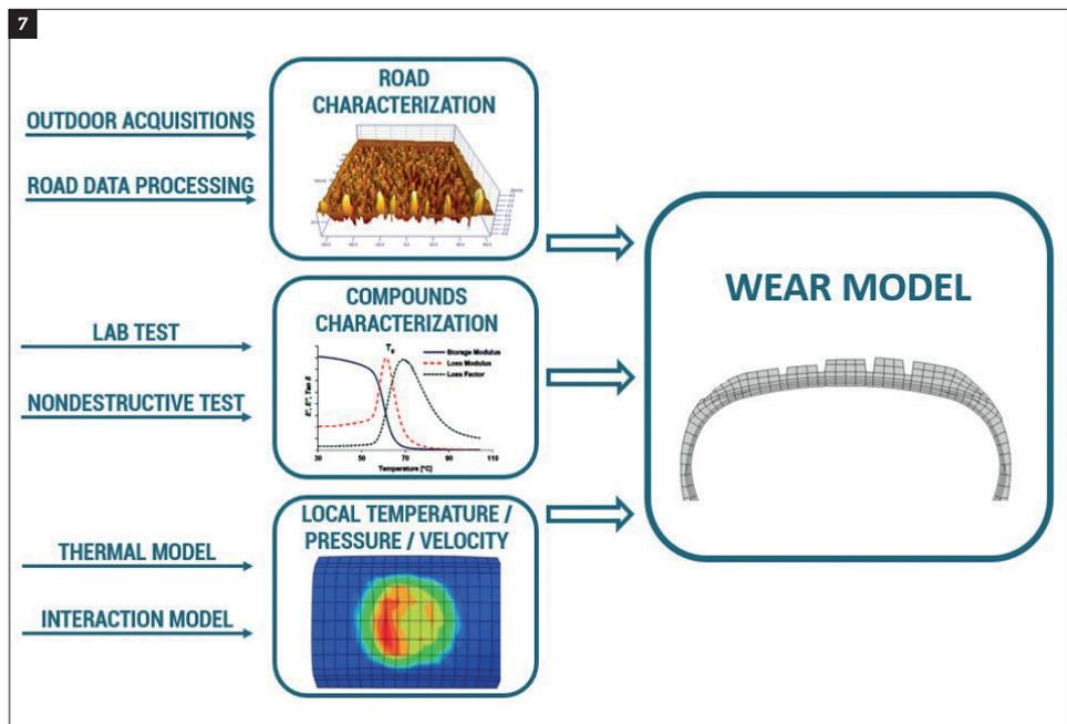
The model takes into account several factors concerning road and tire compound characterization, as well as local thermal phenomena which occur in the contact patch.
